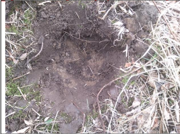
IMAGE 19 COMPLETED TEST PIT
