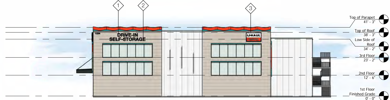
NORTH ELEVATION - BLDG. A Scale: 1" = 30'
