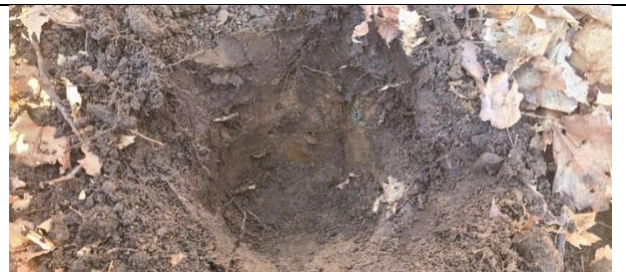
IMAGE 6 VIEW OF TEST PIT IN PROGRESS
