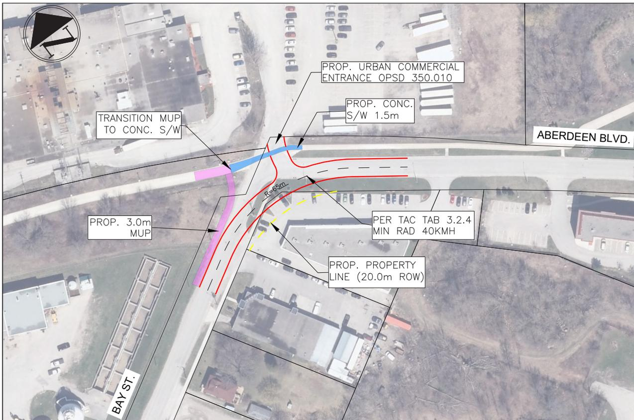
**Figure 5.19** Conceptual design of the recommended re-alignment at Bay Street, Aberdeen Boulevard & TRW Access
