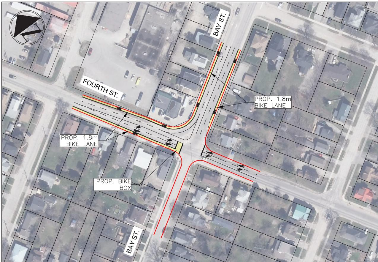
**Figure 5.21** Conceptual design of the recommended signalized intersection layout at Bay Street / Fourth Street with auxiliary turn lanes and cycling facilities
