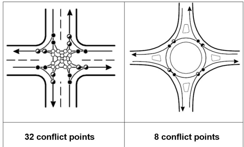
As with any form of intersection control, roundabouts should consider impacts to all users such as pedestrians, cyclists, and transit users. Several objectives within this MTMP revolve around encouraging active transportation and transit usage. The design of intersections and their associated controls have varying impacts to accessibility for these road users that should be considered.
